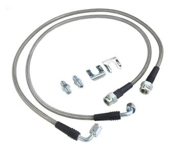
OEM rubber brake hoses generally cannot be adapted to these Wilwood calipers. LSMFG provides braided stainless hoses to go between the caliper and the factory hard line fittings at the chassis. This can be found as an option with the kit ordered, or under Replacement and Additional Parts on the website.
