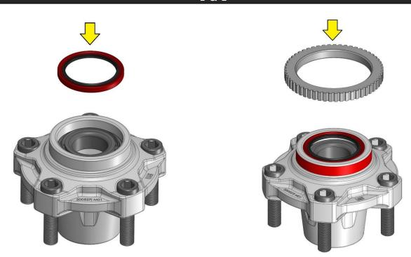
Pack the large inner bearing with high temperature disc brake bearing grease and install into the back side of the hub. The inner seal can then be pressed in or lightly tapped in with a hammer by circling the perimeter. **If your vehicle has front wheel ABS**, remove the reluctor ring from the stock rotor and install it onto the hub.
