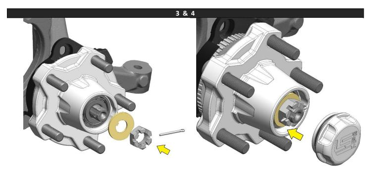
If your vehicle has front wheel ABS, the ABS sensor will be remounted to the spindle in similar fashion as stock. You can now install the hub onto the spindle, then pack the smaller outer bearing with grease and install under the washer, castle nut, and supplied cotter pin. After bending the leg of the cotter pin, install the machined dust cap as shown.
