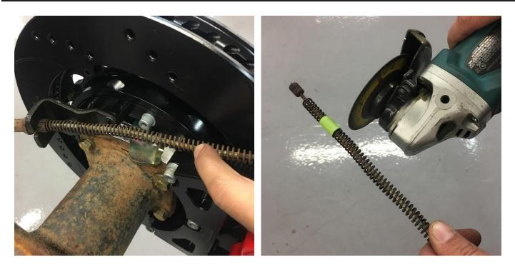
Install the stock parking brake cable into the bracket to hold cable in place. Mark the cable and spring to be cut beyond the cable stop by 1". Use a cut off wheel or cable cutters to cut the cable to the desired length.
