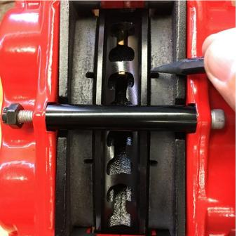
Lubricate the caliper mounting studs with lightweight oil. Initially place one .875x.375x.035 shim on each stud of the bracket. Mount the caliper using lock nuts and washers and ensure that it fully seats on the bracket and does not contact the rotor.
