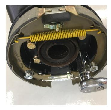
The parking brake assembly can now be installed onto the axle with the supplied hardware. If the kit was optioned with braided hoses, you can position the brake line bracket on the bottom 2 holes of the flange with the tab facing the front side of the axle (NOT pictured). The axle shaft can now be reinstalled per OEM recommendations. NOTE: Your axle may vary from the image shown.
