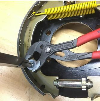
When using the stock parking brake cables, you will need to disassemble the parking brake assembly to install a new cable bracket. Your new levers are included separately. If you purchased our <a href="Parking Brake Cable Kit">Parking Brake Cable Kit</a>, steps 1-9 are **NOT** required. To swap them out, start by removing the retention springs as shown.
