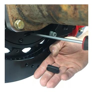
Adjust the parking brake shoes outward using a drum shoe adjustment tool (available at your local parts store) or a flat head screwdriver. You'll do this by spinning the rotor slowly until a slight drag is felt against the hat/drum. The rotor will need lug nuts installed while doing this so that is remains fully seated against the axle shaft. **NOTE:** Your axle may vary from the image shown above.
