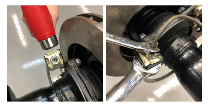
Install the retaining clip as shown, being careful not to bend the hose bracket. The factory brake line can then be repositioned into the top side of the brake line bracket and hose. **Use caution as to not kink the hardline during repositioning.** Next, tighten the brake line nut into your hose. It is best to use a wrench to support the rubber hose from spinning in the key of the hose bracket. **For kits without parking brake calipers, skip to Additional Information and Recommendations.**
