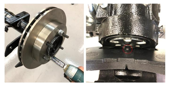
Install the rotor using 2 lug nuts to retain it. **NOTE:** Verify that the rotors are sitting flat against the axle shaft. **Kits with parking brake calipers** should be checked to confirm the pad is seated flat against the piston face, with the boss of the brake pad lining up with the notch in the piston face.
