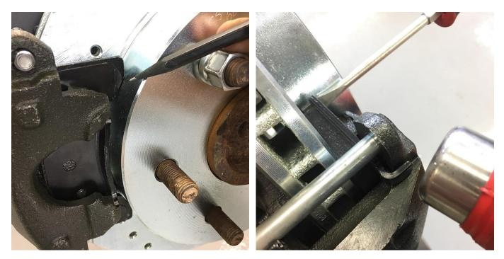
With the caliper bolted into place, check the corners of the pads against the rotor. If there is contact in this spot, you can wedge a flat head screwdriver under the corner and use a hammer to lightly tap the ear of the pad and hold tension away from the rotor. If the pad still contacts the rotor, it may be necessary to lightly sand the corner of the pad until there is adequate clearance. If you installed Wilwood calipers, check this area as well as the body of the caliper to the rotor bell.
