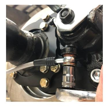
Install the banjo bolt and crush washers into the hose as shown. If your hose has an offset, place the offset side of the fitting **away** from the caliper, then install the hose onto the caliper as shown. (If it is straight, either side can be used). Install the retaining clip being careful not to bend the hose bracket.
