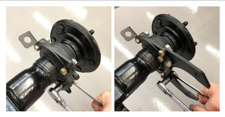
For kits with non-parking brake calipers, bolt on the brackets using the supplied hardware as shown and torque to 20ft-Ibs. Your caliper should be mounted to the REAR (back) of the axle. For kits with parking brake calipers, temporarily leave these bolts loose until the caliper can be bled in the position shown under Parking Brake Caliper Setup.
