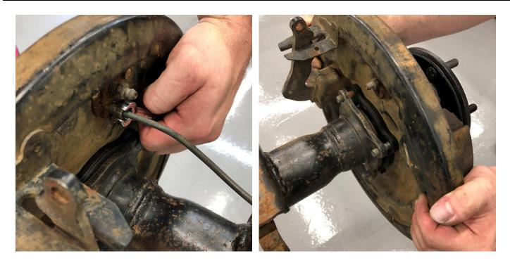
Remove the factory brake line at the back of the drum backing plate. Then remove the 4 nuts securing the axle to the flange. It may be necessary to use a lubricant on these threads. Remove the axle and drum backing plate from the housing.
