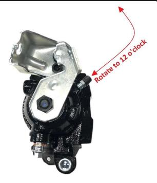
When bleeding this type of parking brake caliper, it is best to temporarily position the caliper so the screw is **vertical to the ground.** If it is not, then it will be necessary to reposition the vehicle, the axle, or the caliper. If **the bleeder screw is not vertical to the ground while bleeding, then you can bleed gallons of fluid through it without eliminating all of the air.**
