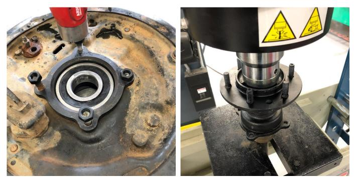
After removing the axle, thread the 4 flange nuts back on flush with the tops of the studs, and remove the studs by driving out with a hammer. This will allow the backing plate to be removed and discarded. Optionally, a new wheel bearing can be installed at this time. The axle can now be reinstalled into the bearing on a press by supporting the bearing as close to the center as possible.
