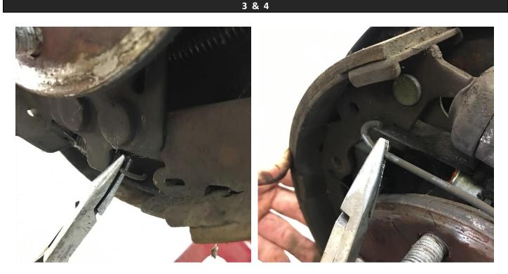
Remove the 2 other retaining springs above and below the axle as shown.
