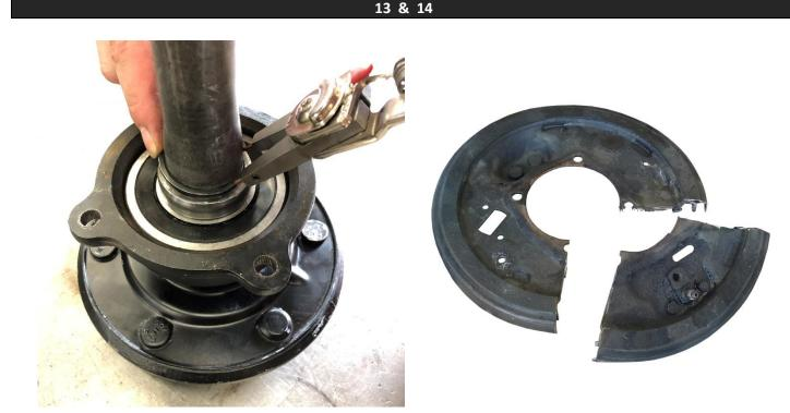
Reinstall the retaining ring, and then install the axle into the housing. **Alternatively to pressing off the bearing:** the user can choose to remove the studs, slip the backing plate down on the axle, then cut a pie shape out as shown using a reciprocating saw or cut-off wheel. When this is done, it is possible to remove the backing plate without removing the bearing from the axle shaft.
