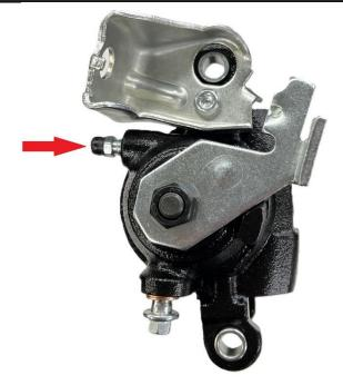
When bleeding this type of parking brake caliper, it is best to temporarily position the caliper, so the screw is **horizontal to the ground**. If it is not, then it will be necessary to reposition the vehicle, the axle, or the caliper. **If the bleeder screw is not parallel to the ground while bleeding, then you can bleed gallons of fluid through it without eliminating all of the air.**
