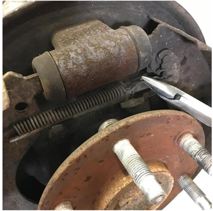
This installation refers to the **passenger side** of the axle. All steps are to be repeated on the driver side. Start by removing the factory drum. It may be necessary use a lubricant around the axle register to do this. Once the drum is removed, remove the first brake shoe retaining springs as shown.
