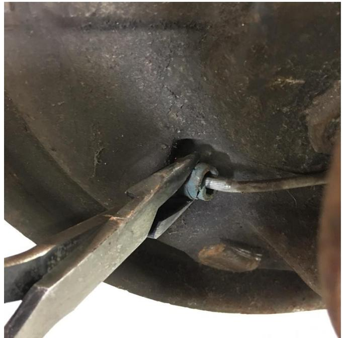
Remove the brake shoes by prying off the retainers on each side. The cable can then be removed from the backing plate by depressing its perimeter springs and pulling it through.
