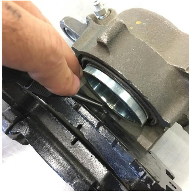
**Kits with non-parking brake calipers** should be checked to confirm the machined pad spacers are present and make sure the notch in the pad spacer lines up with the corresponding boss on the brake pad. If equipped with a pad clip, insert this into the bore.
