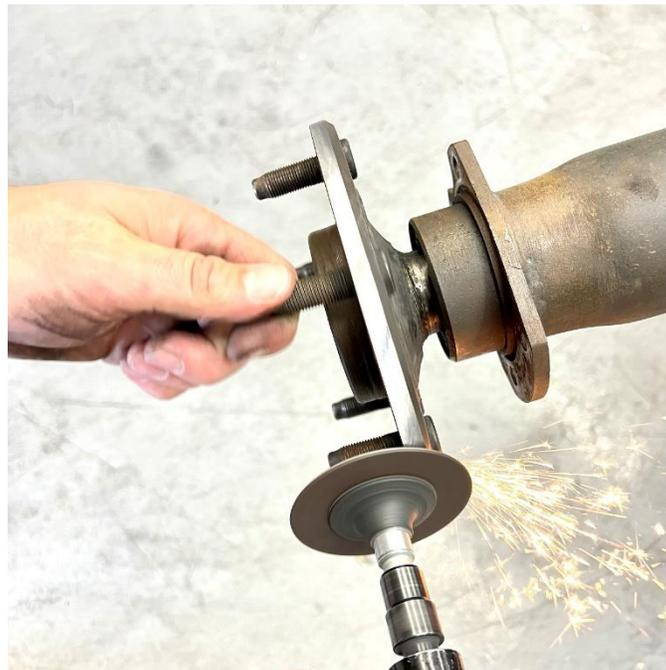
**Normally not required, but in some cases** the OD of the axle shaft flange may be too large to fit inside of the supplied rotor. If this happens, the solution is to simply remove material from the outside of the axle flange with a sander while rotating the shaft as shown.
