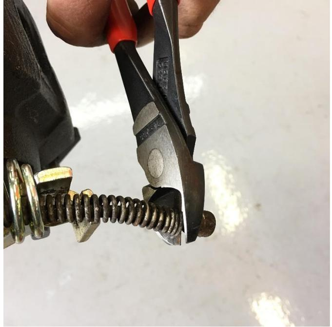
Depending on factory cable lengths, the existing cables can sometimes be used without any modification. If they are too long, then cut off the cable stop as shown using cable cutters or a cut-off wheel. The spring can be removed with the cable installed into the parking brake caliper as shown.
