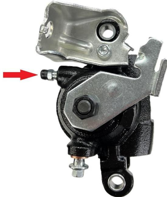
When bleeding this type of parking brake caliper, it is best to temporarily position the caliper, so the screw is **horizontal to the ground**. If it is not, then it will be necessary to reposition the vehicle, the axle, or the caliper. **If the bleeder screw is not parallel to the ground while bleeding, then you can bleed gallons of fluid through it without eliminating all of the air.**
