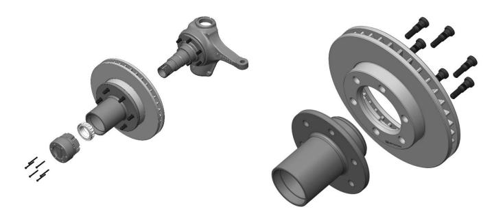
This installation refers to the **passenger side**. All steps are to be repeated on the driver side. For instruction purposes, the knuckle is shown as being removed, but it's not necessary to remove the knuckle to install new brakes. First, remove the stock caliper from the knuckle, then disassemble the hub, spindle, caliper bracket, and remove the stock rotor by pressing out the wheel studs. After the rotor is removed, the stock wheel studs will be pressed back into the hub.
