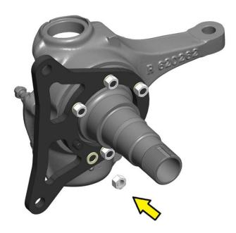
The stock spindle snout can be reinstalled onto the knuckle, followed by the steel intermediate bracket. Install as shown with the provided flat washers and center lock nuts. Torque to 40ft-lbs.
