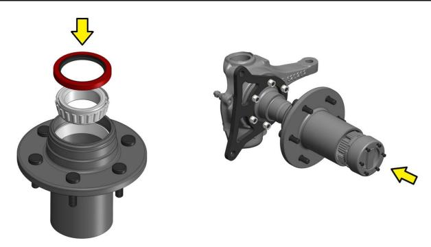
Pack the supplied inner bearing with high temperature disc brake bearing grease and install new seal as shown. Install the hub onto the spindle with greased outer wheel bearing and all factory hardware.
