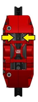
This kit contains distinct right and left-hand calipers that must be mounted in the correct direction. They should be positioned so that the largest pistons are at the rotor exit end of the caliper. Lubricate the caliper mounting studs with lightweight oil. Initially place two .438x1.0x.030 shims on each stud of the bracket. Mount the caliper using lock nuts and washers and ensure that it seats on the bracket and does not contact the knuckle.
