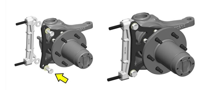
The radial brackets can temporarily be installed at this time using the supplied M14 bolts with flat washers and one spacer washer between the it and the intermediate bracket. It is not necessary to torque them at this time.
