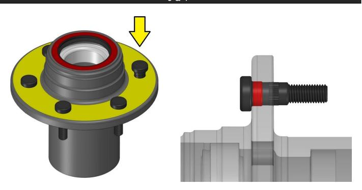
Note that the studs will be pressed past their shoulder (shown here in red) so that the heads seat completely against the flange. A hydraulic shop press will be required for this, with the flange properly supported underneath. Once the studs are reinstalled, a portion of the knurl and shoulder may protrude past the face of the hub.
