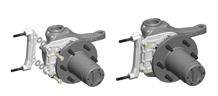
The radial brackets can temporarily be installed at this time using the supplied 7/16 bolts with flat washers and two 1.00x.438x.030 shim washers between it and the intermediate bracket as shown in Step 8. It is not necessary to torque them at this time.
