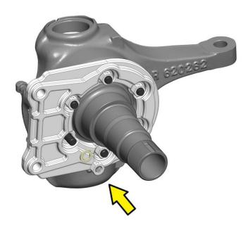
The stock spindle snout can be reinstalled onto the knuckle, followed by the machined aluminum intermediate bracket. Install as shown with the provided flat washers and center lock nuts. Torque to 40ft-lbs.
