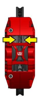
This kit contains distinct right and left-hand calipers that must be mounted in the correct direction. They should be positioned so that the largest pistons are at the rotor exit end of the caliper. Lubricate the caliper mounting studs with lightweight oil. Initially place two .438x1.0x.030 shims on each stud of the bracket. Mount the caliper using lock nuts and washers and ensure that it seats on the bracket and does not contact the spindle.
