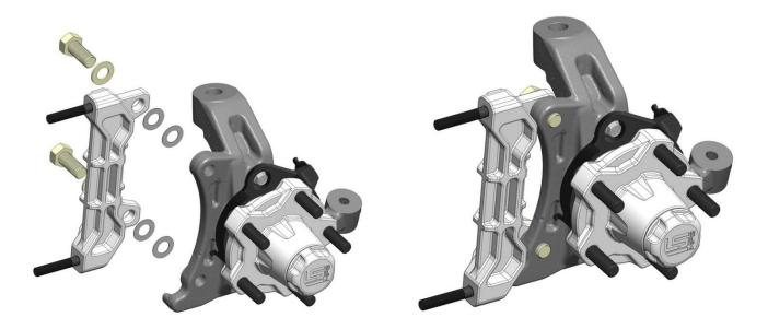
The radial bracket can temporarily be installed at this time using the supplied bolts with flat washers and two .438x.750x.030 shim washers between the bracket and spindle. It is not necessary to torque them at this time.
