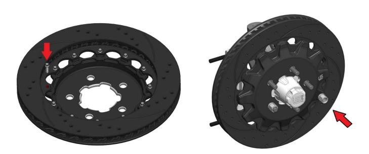
Arrange the rotor and hat in the position shown ensuring the arrow noting rotation direction is correct for its position on the vehicle. Note that the hat should be installed on the flat side of the rotor. Start the first few threads of all 12 of the 5/16-18 x .875 bolts. Using an alternating sequence, apply red Loctite® 271 to the threads, and torque to **25 ft-lbs**. The rotor can be installed on the hub at this time using two lug nuts to hold the hat flat against the hub.
