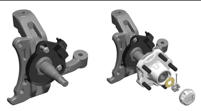
If your truck has front wheel ABS, the ABS sensor will be remounted to the spindle using the bolt hole it previously used on the dust shield. You can now install the hub onto the spindle, then pack the outer bearing (A3) with grease and install under the factory washer, castle nut, and supplied cotter pin. After bending the leg of the cotter pin, install the machined dust cap as shown.
