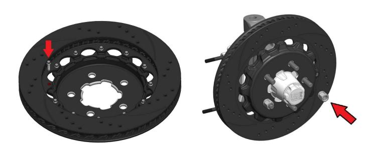
Arrange the rotor and hat in the position shown ensuring the arrow noting rotation direction is correct for its position on the vehicle. Note that the hat should be installed on the flat side of the rotor. Start the first few threads of all 12 of the %-20 12-point bolts. Using an alternating sequence, apply red Loctite® 271 to the threads, and torque to 155 in-lbs. The rotor can be installed on the hub at this time using two lug nuts to hold the hat flat against the hub.
