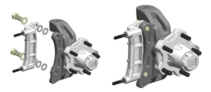
The radial bracket can temporarily be installed at this time using the supplied bolts with flat washers and two .750x.438x.030 shim washers between the bracket and spindle. It is not necessary to torque them at this time.
