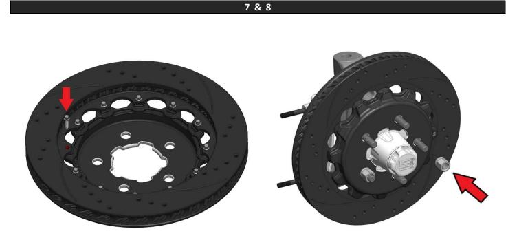
Arrange the rotor and hat in the position shown ensuring the arrow noting rotation direction is correct for its position on the vehicle. Note that the hat should be installed on the flat side of the rotor. Start the first few threads of all 12 of the ¼-20 12-point bolts. Using an alternating sequence, apply red Loctite<sup>®</sup> 271 to the threads, and torque to **155 in-lbs**. The rotor can be installed on the hub at this time using two lug nuts to hold the hat flat against the hub.
