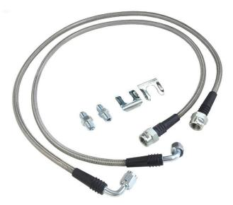
OEM rubber brake hoses generally cannot be adapted to Wilwood calipers. These Wilwood calipers utilize a 1/8 NPT fitting. **DO NOT** thread any OEM tube-nuts into the caliper directly without adapting to 1/8 NPT.
